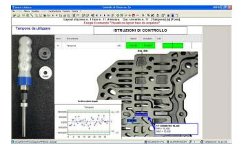
Example of operator interface with option Lay Out Designer, which allows to personalize the display for each phase of the control cycle.
