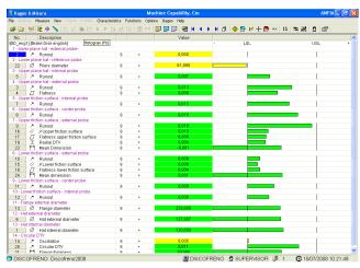
User interface totally configurable: simple and immediate, with the global result of the test (green for good, red for reject and yellow for uncertain), punctual values for each characteristic of the control plan and possibility to display up to 6 graphics for the critical sections.
