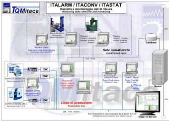
Example of a structure for the data collection with metrological room, production line, quality department, database on a server, monitoring with direct interaction on work stations.
