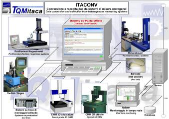
Example of instruments (with PC and with files generation) which can be interfaced using Itaconv 6.
