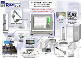
Example of instruments which can be interfaced to a SPC Itastat Measure station.
