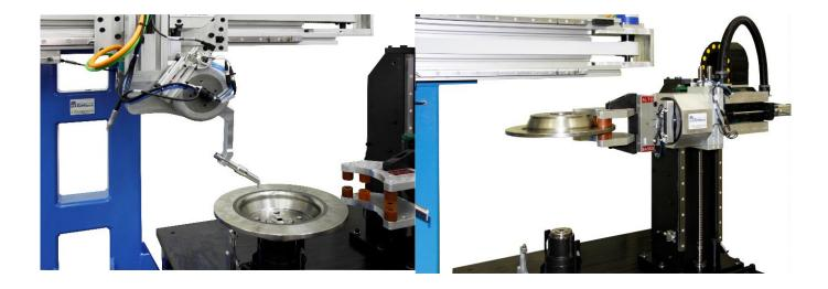
If it is necessary to control also the support plane, the bench will be equipped with an automatic tilter.
