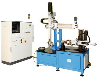
Automatic station for 100% cracks control on brake discs and brake drums
