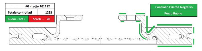
Example of a screen in case of a disc with a crack detected on the upper braking surface. Rejected piece
