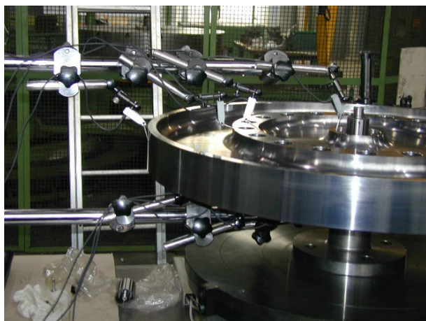
Itageo 6° integrated on a machine designed Ad Hoc for the control of turbine rotors.
