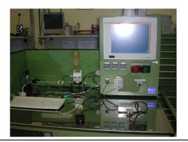
Station for the control at the end of line of aerosol machines.
