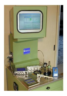
Example of a SPC station out of line, in heavy carpentry, with support shelf in stainless steel, operator keyboard in stainless steel, 8 buttons, electrical and ventilation system according to CE rules. Standard PC and UPS. Interface for manual instruments (electronic probes, vernier calipers, pneumatic gauges, etc...).
