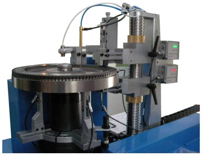
In the picture above note the laser sensor completely closed in a protection with automatic gate, with pneumatic activation, which assures the respect of the requested safety standards.
