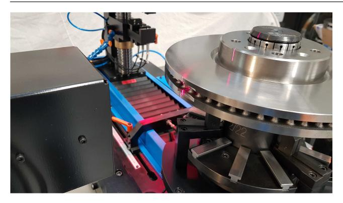
TQM Itaca Technology develops modular solutions to be installed on measuring stations in order to perform the external surface control to identify the presence of defects, for example on Brake Disc (pitting, pores, lack of material, defects coming from foundry process etc.) after the machining and balancing phases.
