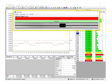
At the end of the test, that is performed during the normal functioning cycle of the station, the software will send information to <u>ITAGEO</u> (after an initial brief setup for defect size and balancing feature detail) about the part classification on GOOD or REJECTED. The data of this attribute characteristic is saved together the other measures in the database.
