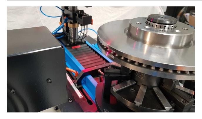
TQM Itaca Technology develops modular solutions to be installed on measuring stations in order to perform the external surface control to identify the presence of defects, for example on Brake Disc (pitting, pores, lack of material, defects coming from foundry process etc.) after the machining and balancing phases.
