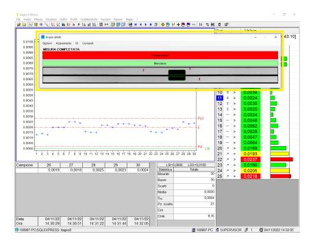
At the end of the test, that is performed during the normal functioning cycle of the station, the software will send information to <a href="ITAGEO">ITAGEO</a> (after an initial brief setup for defect size and balancing feature detail) about the part classification on GOOD or REJECTED. The data of this attribute characteristic is saved together the other measures in the database.
