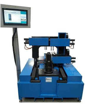
TQM Itaca Technology has developed a dedicated measuring system for brake disk and drums that performs automatic re-tooling of the measuring probes on the bench.
