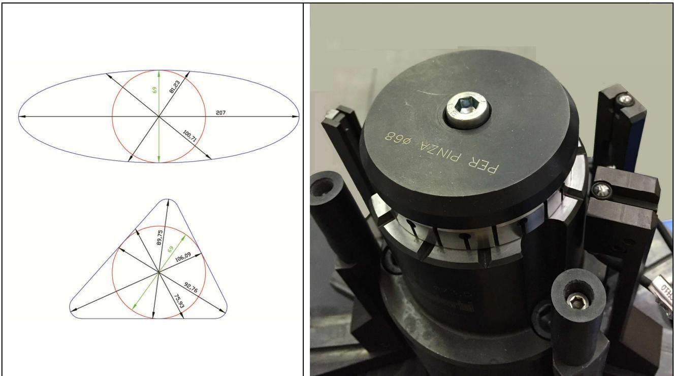
The solution patented by **TQM ITACA TECHNOLOGY srl** simulates the mounting condition; so the measurement made is correct and independent from the bore form.
