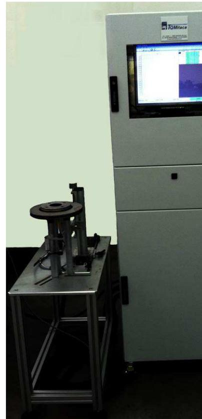
There are also available stations for FRF control directly integrated in the **Itageo 6<sup>®</sup>** gauge: there is an elevator which has the function of release the disc from the gauge for the control of frequencies and, in the meanwhile, it allows to avoid the direct load of the disc on the precision mandrel made by the load/unload robot.
