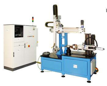
Automatic station for 100% cracks control on brake discs and brake drums
