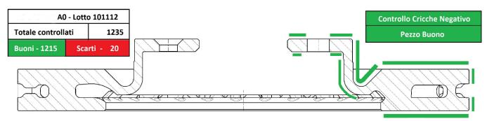
Example of a screen in case of a disc with a crack detected on the upper braking surface. Rejected piece
